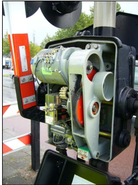
Photo 5: The mechanism inside the barrier unit.
