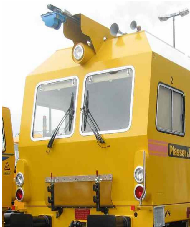
Picture 1: Ballast Profile Measuring System Fitted to a Plasser EM-SAT System
