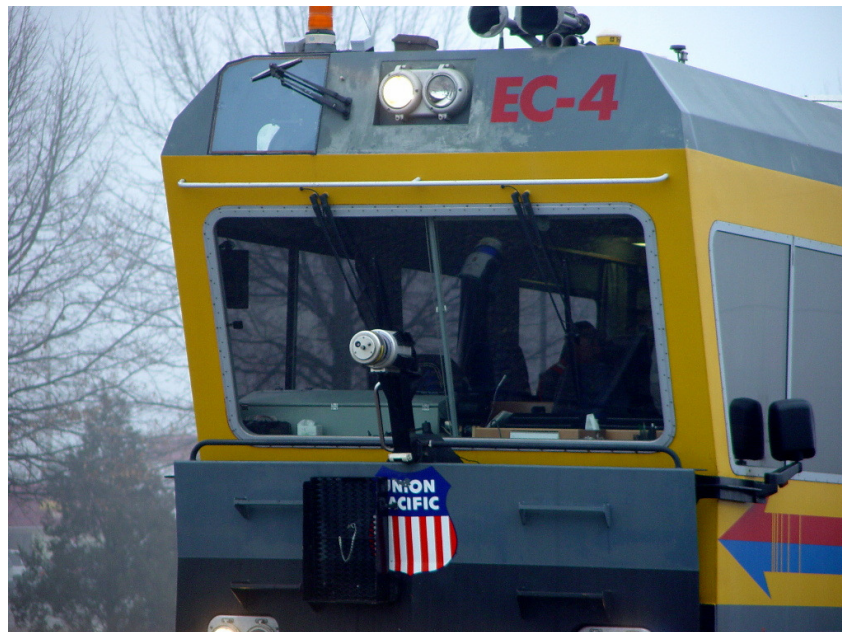
Picture 2: Ballast Profile Measuring System Fitted to Union Pacific Inspection Train
