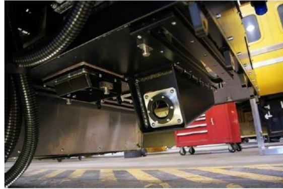
Plain Line Pattern Recognition camera
